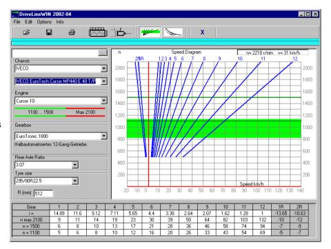
**DrivelineWIN** is mainly used for trucks and buses, but it is also possible to calculate such diagrams for passenger cars.
